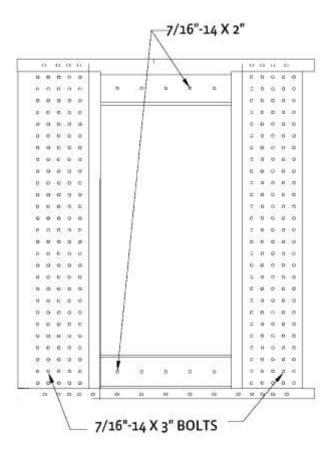
Before installing the outer protective weather door cover, verify that the mounting hinges are installed as shown in the following illustrations. Install foam sealant on interior of the door protective weather cover where the cover will close against the exterior door frame.
