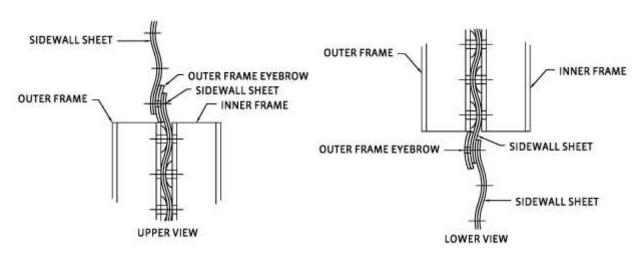
For 2 and 3 stiffened bin designs,  $7/16-14 \times 3.0^\circ$  bolts with the heads located on the exterior of the bin will be used in the left and right channels at the locations shown below, and  $7/16-14 \times 2.0^\circ$  bolts with the heads located on the exterior of the bin will be used in the top and bottom channels at the locations shown below.
