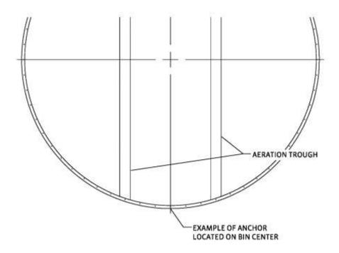
**Important Note:** Do not install the expansion type anchor bolts inside the aeration trench at this time.
