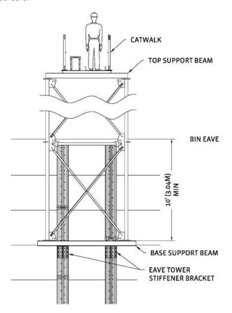
The following illustrates the roof height of various models to assist in selecting the correct height of eave tower support.
