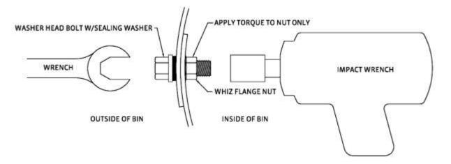
Please note the following wrench / socket size to be used on the corresponding hardware:
