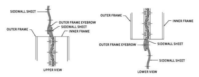
For 2 and 3 stiffened bin designs,  $7/16-14 \times 3.0^{\circ}$  bolts with the heads located on the exterior of the bin will be used in the left and right channels at the locations shown below, and  $7/16-14 \times 2.0^{\circ}$  bolts with the heads located on the exterior of the bin will be used in the top and bottom channels at the locations shown below.
