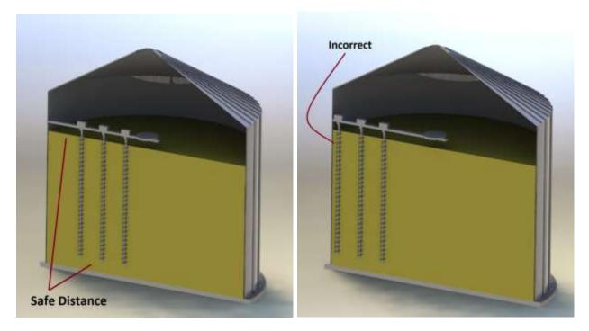
Down augers may require shortening in order to provide minimum floor clearance of 3"-5" (76mm -127 mm) or additional clearance for sweep augers. Always follow the manufacturer down auger shortening procedure.
