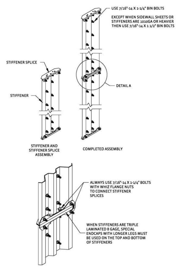
5. Loosely assemble ring #3 following the <u>sidewall and stiffener installation instructions</u>. Refer to the <u>gauge charts</u> for the correct gauge of material to use. Using a large alignment punch, force the stiffeners upward so the splices are tightly compressed (blocks may also be used to compress the stiffener splices). Tighten 4 bolts in ring #3 to keep the stiffeners compressed. Loosely install the stiffener splice plate hardware.
