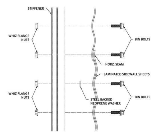
On bins with single sidewall sheets on the bottom ring, install steel-backed neoprene washers between the bottom 2 ring stiffener and the sidewall sheets on the bottom 2 holes as shown in the following illustration. The neoprene rubber side of the washer should contact the sidewall sheet.
