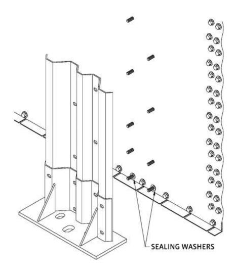
On bins with laminated sidewall sheets on the bottom ring, install steel-backed neoprene washers between the bottom 2 ring stiffener and the sidewall sheets on <u>all holes</u> as shown in the following illustration. <u>The neoprene rubber side of the washer should contact the sidewall sheet</u>.
