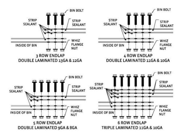
Lap the sheets so that when located outside the bin, facing toward the bin, the right end of each sheet is always on the outside of the bin and the left end is always on the inside.
