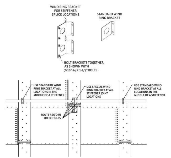
**Important Note:** All wind ring segments are 248" (629.92cm) long, and may require a field cut to keep couplers in between the wind ring brackets.
