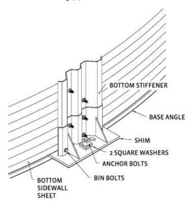
If anchor bolts are not pre-formed as stated above, and the anchor bolt radius is not held, the bins warranty will be nullified. All anchor bolts must project a minimum of 2" (5.08cm) above the concrete floor. It is recommended to keep anchor bolt projection to a maximum of 3" (7.62cm) above the concrete.
