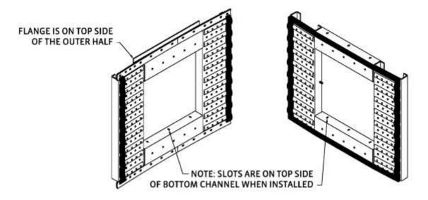
Bolt the inner and outer frame to the bin sidewall with  $7/16-14 \times 3.0$ " bin bolts, making sure to only place bolts in the holes shown in the following illustrations. The top eyebrow on the outer frame is to be placed behind the sheet above the door. The bottom eyebrow is to be placed on the outside of the sheet below the door. Bolt the upper and lower channel frame together with  $7/16-14 \times 2.0$ " bin bolts and whiz flange nuts.
