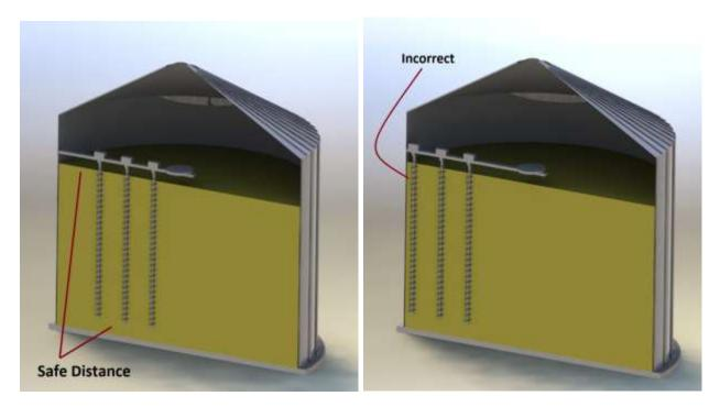
Down augers may require shortening in order to provide minimum floor clearance of 3"-5" (76mm -127 mm) or additional clearance for sweep augers. Always follow the manufacturer down auger shortening procedure.
