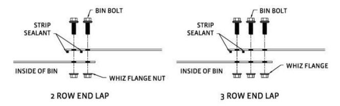
Sealant is required at specified seams for a watertight seal. Wipe off the outside ends of all the sidewall sheets to remove excess oil so that the sealant will adhere to the metal. Place the sealant as near as possible to the vertical inside edge of the sidewall sheet at every vertical seam.
