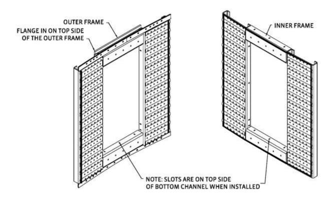
Bolt the inner and outer frame to the bin sidewall with  $7/16-14 \times 3.0$ " bin bolts, making sure to only place bolts in the holes shown in the following illustrations. The top eyebrow on the outer frame is to be placed behind the sheet above the door. The bottom eyebrow is to be placed on the outside of the sheet below the door. Bolt the upper and lower channel frames together with  $7/16-14 \times 2.0$ " bin bolts and whiz flange nuts.
