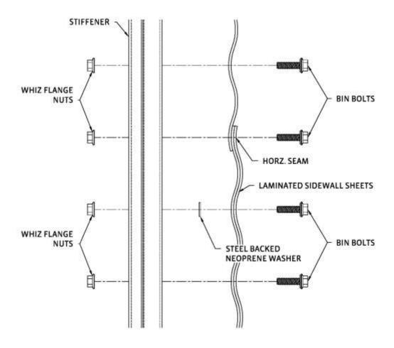
On bins with single sidewall sheets on the bottom ring, install steel-backed neoprene washers between the bottom 2 ring stiffener and the sidewall sheets on the bottom 2 holes as shown in the following illustration. The neoprene rubber side of the washer should contact the sidewall sheet.
