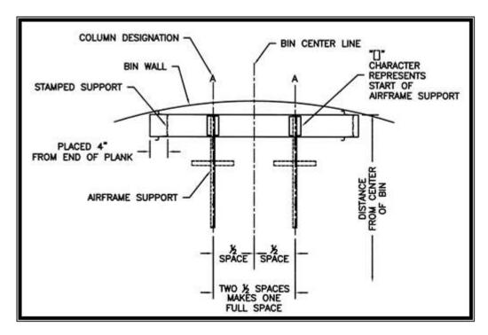
Continue to add airframe support columns and channel lock rows per bulletin 1050-A. The "[]" character specifies the starting position of every Airframe support to be added. Continue to add stamped supports to the end of channel lock rows at a distance of 4" when required, and add a stamped support at splice locations for split floors.
