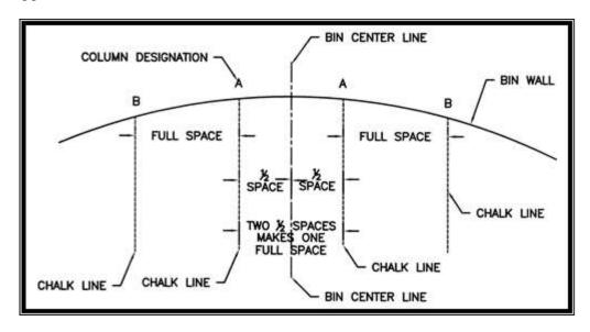
For each half of the bin run additional chalk lines incrementally at the support full spacing dimension. The second location is labeled Column "B". The airframe support column locations continue until the last "alpha" character has had a chalk line established.
