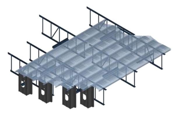
First use the packing list in the full floor bolt bag assembly to verify all floor component parts are present and quantities are correct. Next review the floor support layout for your installation that is based upon the bin diameter, maximum peak grain depth and type of aeration floor (1 piece or split floor). **Note:** For bins 33'-42' (10.05m-12.80m) diameter, floors may be purchased as 1-piece or split floor.
