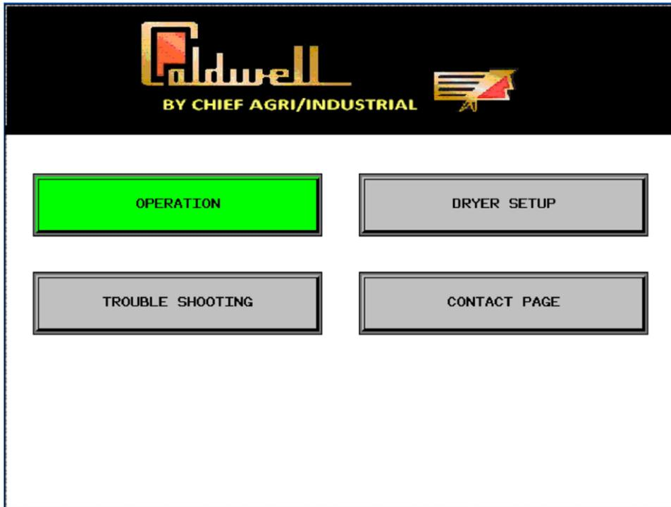
**Operations Screen** – During dryer operation the operations screen will be the main screen referenced unless you are using a DryerMaster unit. In that case you may use the DryerMaster Screen.
