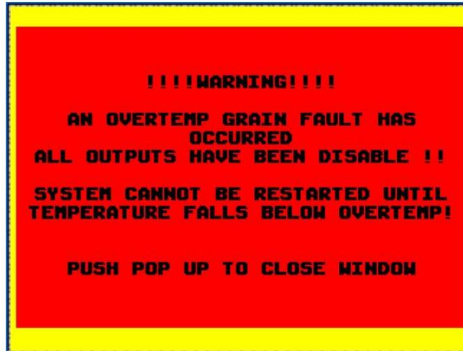
Once the dryer shutdown fault has occurred, the entire drying operation will be shut-down, including the fans, due to the possibility of a grain fire being present. The fault will remain present until all the grain temperature sensors detect a temperature below the high limit setting.
