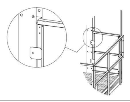
**Note**: Each walk around system consists of (3) end enclosures and (1) gate. The gate can be located in multiple locations as shown in the following illustration.
