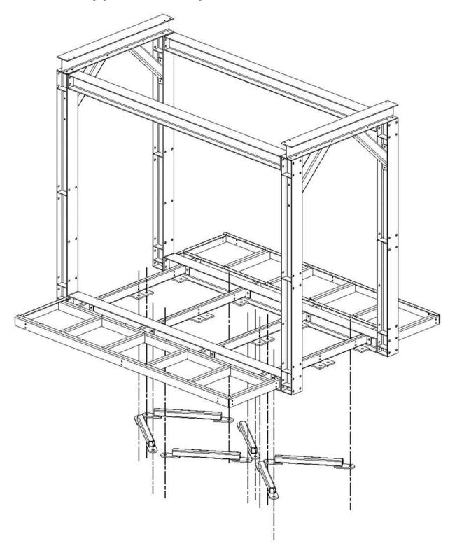
Install the floor zee clips on the floor cross braces using 1/2" x 3-1/2" bolts. **Note**: Leave these connections finger tight at this time.
