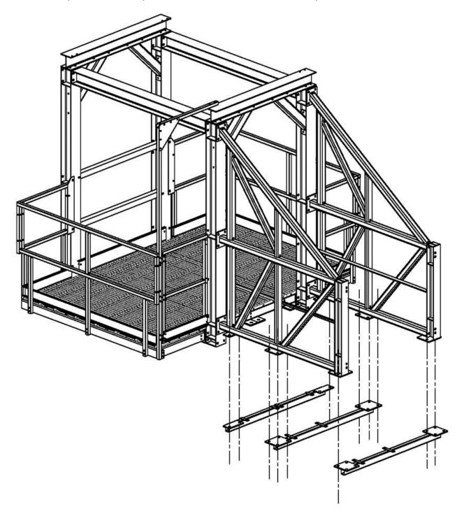
Install wind diagonals on the cross/end braces using 3/4" x 2-1/2" bolts. The attachment of the wind diagonals will align with the bottom side of the attachment plate on the cross/end braces.
