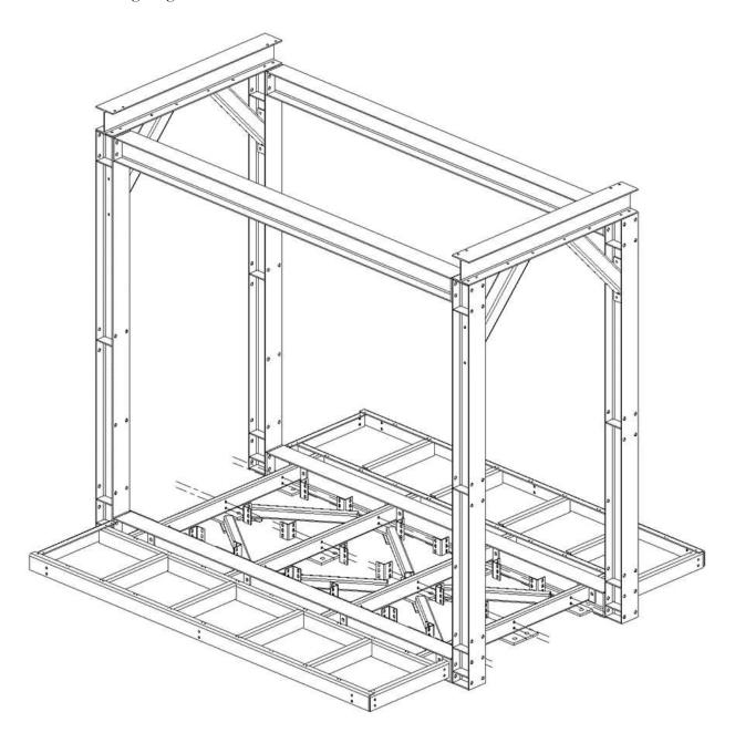
Attach the floor zees to the floor zee clips using 1/2" x 1-1/4" bolts. Verify the top of the floor zees are at the same level as the top flange of the bottom beam and fully tighten floor connections.
