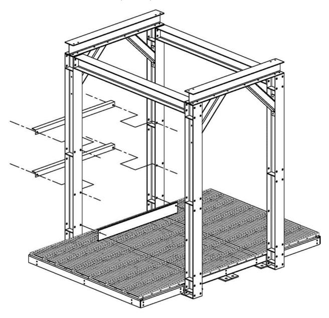
Attach the side and end handrails to the platforms using 1/2" x 2-1/2" bolts.
