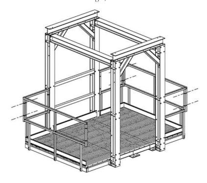
Attach the end handrail support to the vertical column using 3/4" x 1-1/2" bolts. Attach the end handrail support to the end handrail using 1/2" x 2-1/2" bolts.
