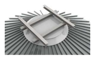
Locate the walk around over the support beams. Verify the support beams span two bottom walk around beams. Verify the support beams are contacting the bottom walk around beams only and are <u>not</u> supported by or welded to any other bracing. Support beams must be fully welded at all contact points with 1/4" (.63cm) fillet weld.
