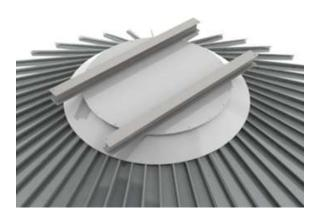
Position intermediate support beams perpendicular to the base support beams. These beams will be perpendicular to the installed walk around and catwalk. **Note**: Verify the height position underneath the catwalk walk around is correct and adjust any peak support posts as required to maintain correct height.
