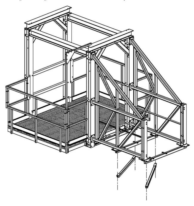
Install the walkway on the slotted tabs located on the cross/end braces using 5/16" x 1-1/2" carriage bolts with diamond washers and whiz flange nuts.
