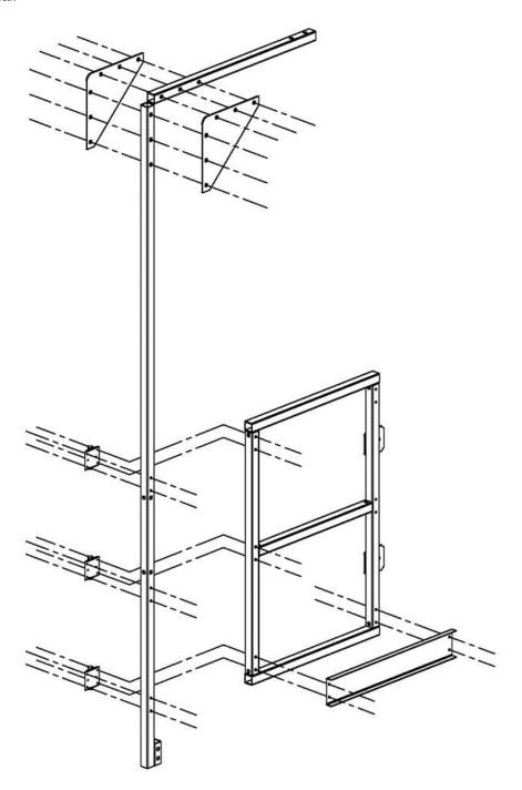
Attach the gate assembly to the platform base using 1/2" x 2-1/2" bolts. Attach the top of the gate assembly to the side handrail using 1/2" x 4" bolts.
