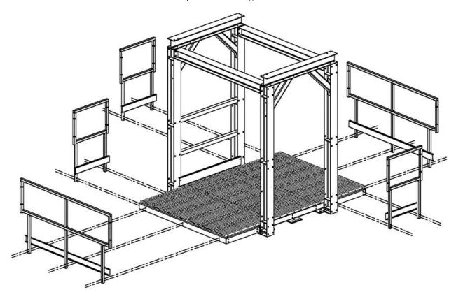
Bolt the end handrails to the side handrails using 1/2" x 4" bolts.
