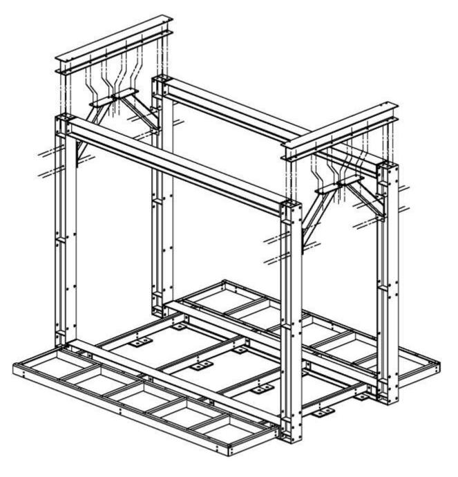
Install the floor diagonal braces to the floor cross brace connection plates using 1" x 2-3/4" grade 8 bolts with lock washers and nuts.
