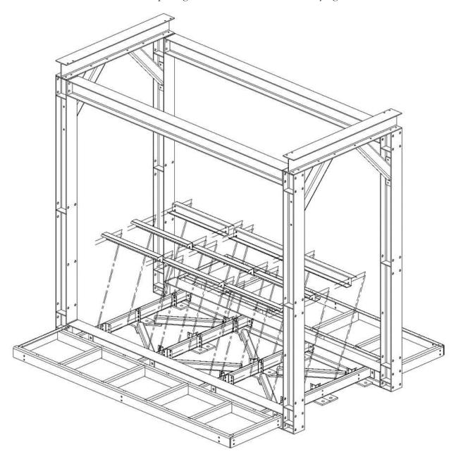
Attach rows of planking to the platform and also the center section using TEK screws. **Note**: Planking is fastened from the underside of the platforms thru the floor zee.
