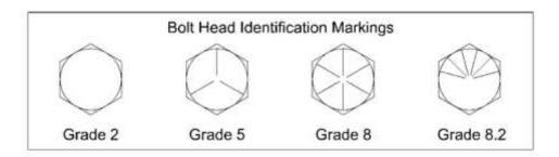
If these descriptions do not correspond with the bolts shipped with the bin, please contact the customer service department immediately. Substitution of any other type or bolt grade or hardware from other sources is not allowed and will void the warranty.
