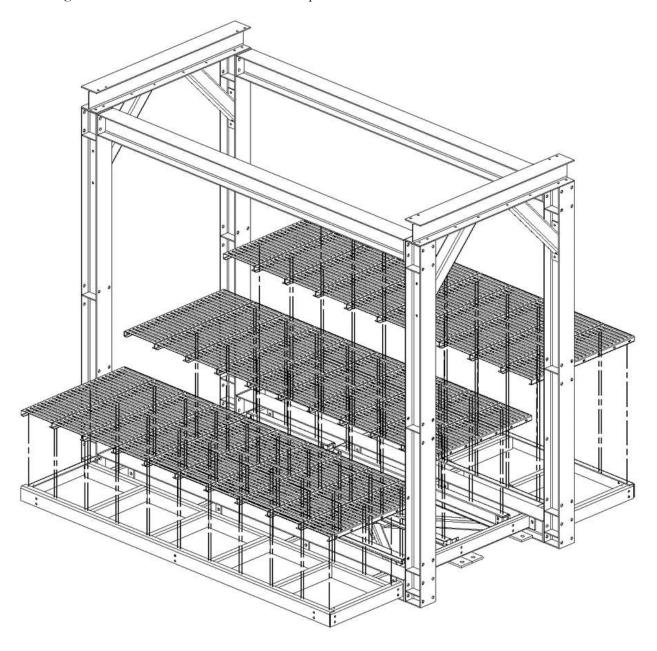
Attach (2) top/mid rail angles to the vertical columns with 3/4" x 1-1/2" bolts. Attach the end toe board to the vertical columns with 1/2" x 2-1/2" bolts.
