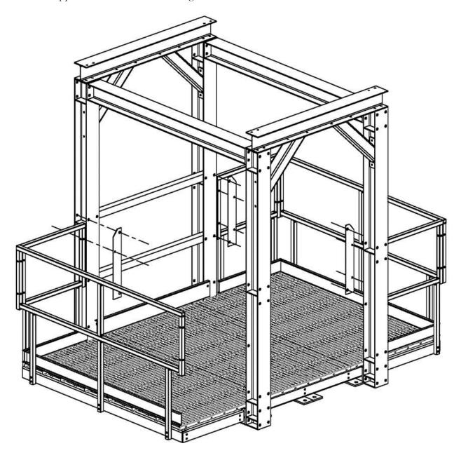
Assemble the gate and gate post as shown in the following illustration. Attach the gate post gussets to the gate post weldment and the gate post cross tube using 1/2" x 2-1/2" bolts.
