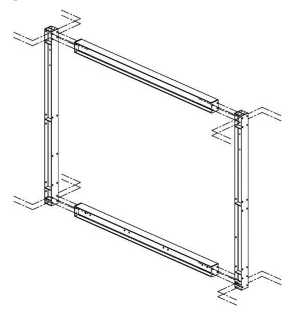
Place the platforms and the floor cross braces between the beam assemblies as shown in the following illustration. Attachment plates on the floor cross braces will align with the holes in the bottom beams. Install the platform/floor brace connections using 3/4" x 2-1/2" bolts.
