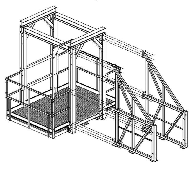
On the end of the truss sides attached to the vertical beam, attach the terminating end member to the bottom of the truss sides with 3/4" x 2" bolts. In the middle of the truss sides, attach the cross brace to the bottom of the truss sides with 3/4" x 2" bolts. On the end of the truss sides attached to the catwalk, attach the standard cross brace to the bottom of the truss sides with 3/4" x 2" bolts.
