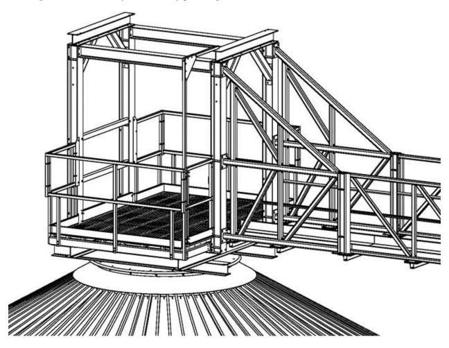
Position base support load beams on the bin peak, parallel to the overall length of the catwalk. Fully weld at all contact points with 1/4" fillet weld.
