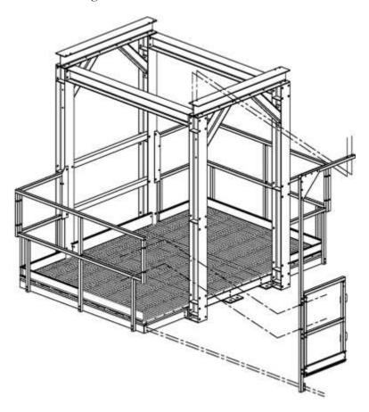
**Note**: If a gate entrance is not required, field drill the column flange and securely bolt the gate closed as shown.
