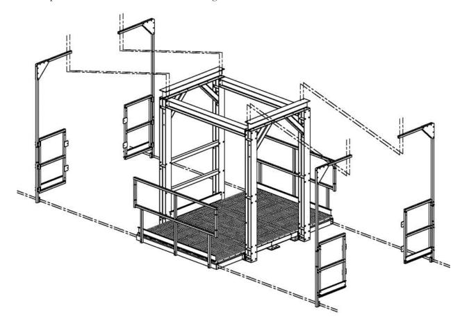
Attach each side truss to the vertical columns using 3/4" x 2" bolts.
