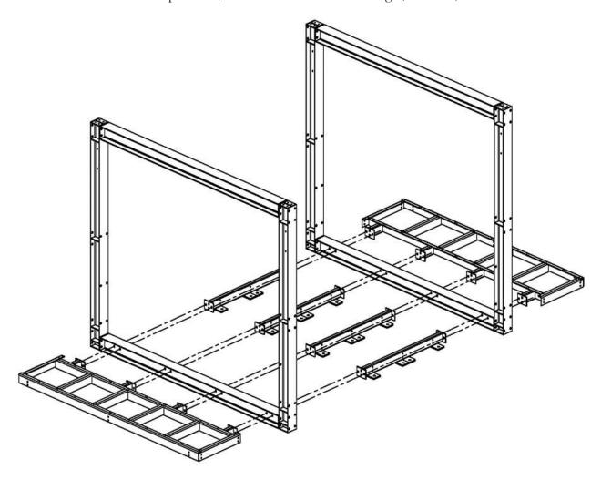
Bolt the ends of the top cross beam to the top of the vertical columns using 1/2" x 1-1/4" bolts as shown in the following illustration.
