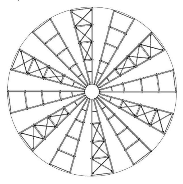
Next, after all the A-frame rafter bays are installed, begin installing the remaining ring segments and bracing.
