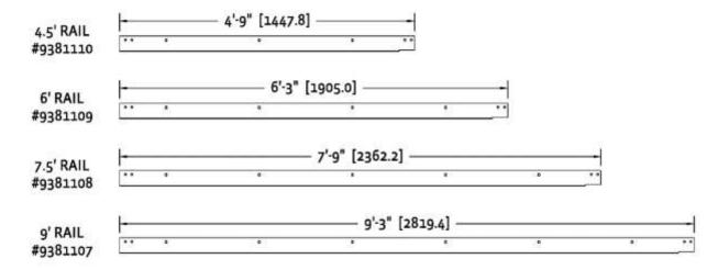
Attach the roof ladder rails to the roof panels by field drilling holes into the vertical rib of the roof panel. Secure the working ring brackets with 5/16" x 3/4" (.79x1.90cm) bin bolts. Roof ladder rungs will then be attached to the roof ladder rails and secured with 5/16" x 3/4" (.79x1.90cm) bin bolts.
