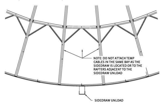
For bins 15 rings and shorter, install the temperature cable brackets as shown in the following illustration. Then attach the temperature cable eye bolt to the rafter using the temperature cable manufacturer's instructions.
