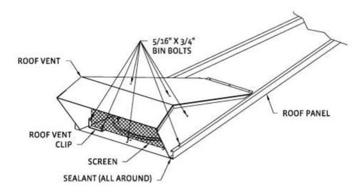
Locate the roof vent assembly on the roof panel (over the manhole) by aligning the holes in the clips with the corresponding holes in the lower end of the roof panel. Mark the outline of the roof vent with a marking pencil so that the vent can be returned to the same position after the caulking is applied.
