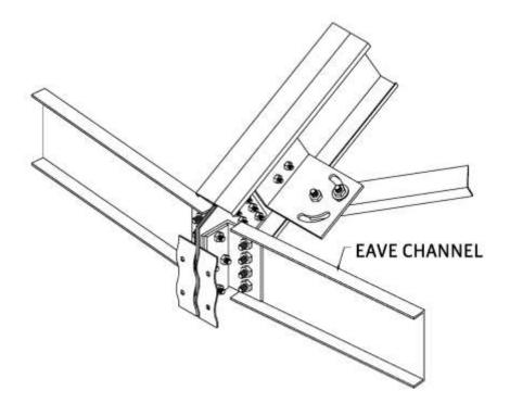
After all the A-frames are built, equally space and attach 4 frames to the peak ring and sidewall. Next attach a left hand and right hand eave bracket to the interior of the top sidewall sheet behind the 2 ring top stiffener using 7/16" x 1-1/2" (1.11x3.81cm) bin bolts with the bolt head located on the interior of the bin, as shown in the following illustration.
