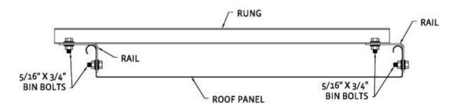
Working up from the roof eave to the roof peak, the rails will need to be overlapped when transitioning from 1 section of rails to the next. Overlap these rails as shown in the following illustration and secure the rails with 5/16" x 3/4" (.79x1.90cm) bin bolts.
