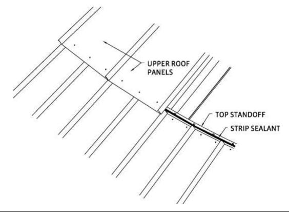
Place sealant on the roof panel flashing extensions where the top end of the upper roof panel will contact the flashing. Attach the top end of the roof panel with 5/16" x 3/4" (.79x1.90cm) bin bolts with the bolt heads located on the exterior of the bin roof panel. Verify that the upper roof panel rib is aligned with the center of the roof rafter.
