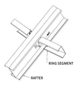
Located at the eave, looking upward towards the peak, verify the position of the ring segment on the clip is correct according to its position on the rafter. Verify the correct bolt size is used in the ring segments.
