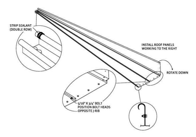
As each roof panel is set into place, insert an alignment punch through the hole in the rib at the bottom of each roof panel. Temporarily clamp the two roof panels together with vise grips so that the punch can be removed. Insert a 5/16" x 3/4" (.79x1.90cm) bolt and only hand tighten the hardware at this time.
