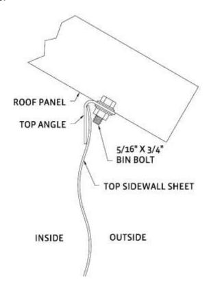
Install roof panels in a counter clockwise direction, always working to the <u>right</u> around the bin. Place sealant on the top right rib of the previously installed roof panel. Position the roof panel in a vertical position and lock the left rib of the current panel over the right rib of the previously installed panel. Slowly rotate the roof panel down.
