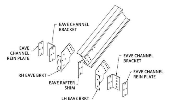
Attach the eave channels to the eave channel clip using 3/4"x2" (1.90x5.08cm) bolts.
