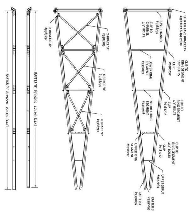
Attach the ring segment clips to every rafter as shown in the following illustration. Ring segment clip 9383737 requires 1/2" x1-1/2" (1.27x3.81cm) bolts.
