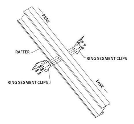
Attach the ring segments to the ring segment clips as shown in the following illustration.
