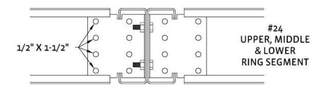
Attach the upper roof struts between every rafter as shown in the following illustration. Upper struts use 1/2"x1-1/2" (1.27x3.81cm) bolts.
