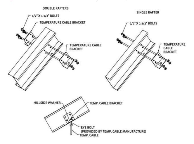
For bins 16 rings and higher, install the temperature cable brackets as shown in the following illustration. Then attach the temperature cable support beams to the bottom of the roof rafters, using pipe spacers as needed when roof x bracing interferes with the temperature cable beams. Then attach the temperature cable eye bolt to the support beam using the temperature cable manufacturer's instructions.
