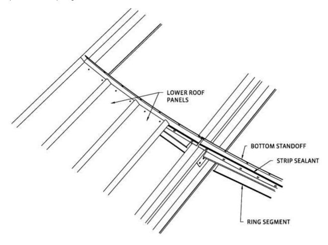
**Important Note**: Verify that the roof panel rib is aligned with the rafter centerline.
