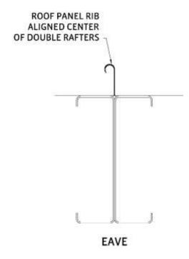
As each roof panel is set into place, insert an alignment punch through the hole in the rib at the bottom of each roof panel. Temporarily clamp the two roof panels together with vise grips so that the punch can be removed. Insert a 5/16° x 3/4° (.79x1.90cm) bolt and only hand tighten the hardware at this time.
