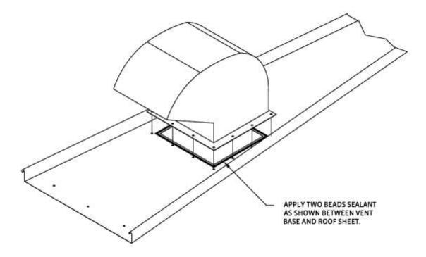
The pre punched roof panels may be located in 3 separate locations and are required to be equally spaced around the bin during the roof installation. In addition to being equally spaced, the vents must be staggered correctly in 3 locations.
