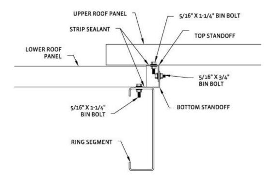
Place sealant on the top side of the top standoff angle where upper roof panels will be attached.
