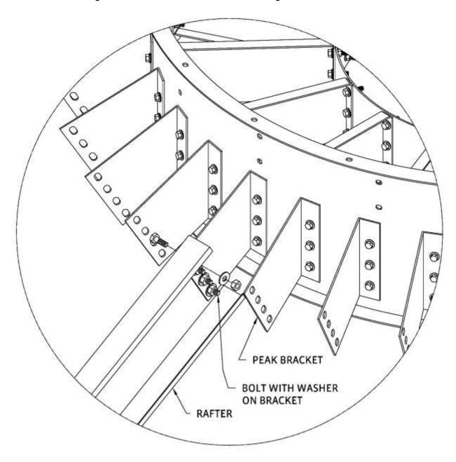
Once the 4 initial A-frames are installed verify that the peak ring is level, then continue installing the remaining A-frame rafter bays.
