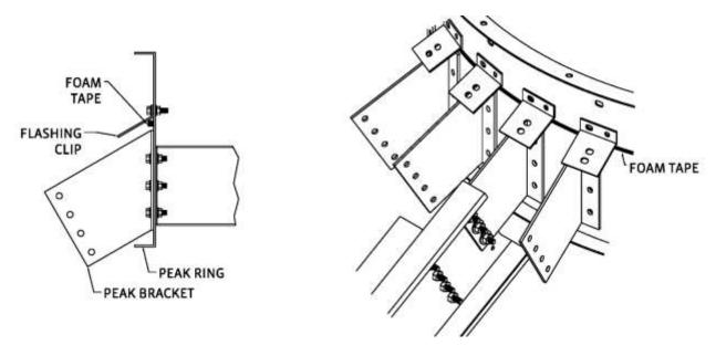
Install the roof panel flashing extensions as shown in the following illustrations. These extensions are installed in a clockwise pattern around the peak with 7/16" x 1-1/4" (1.11x3.17cm) bin bolts. The first flashing extension must be centered on the roof rafter and the flashing clip on the peak ring.
