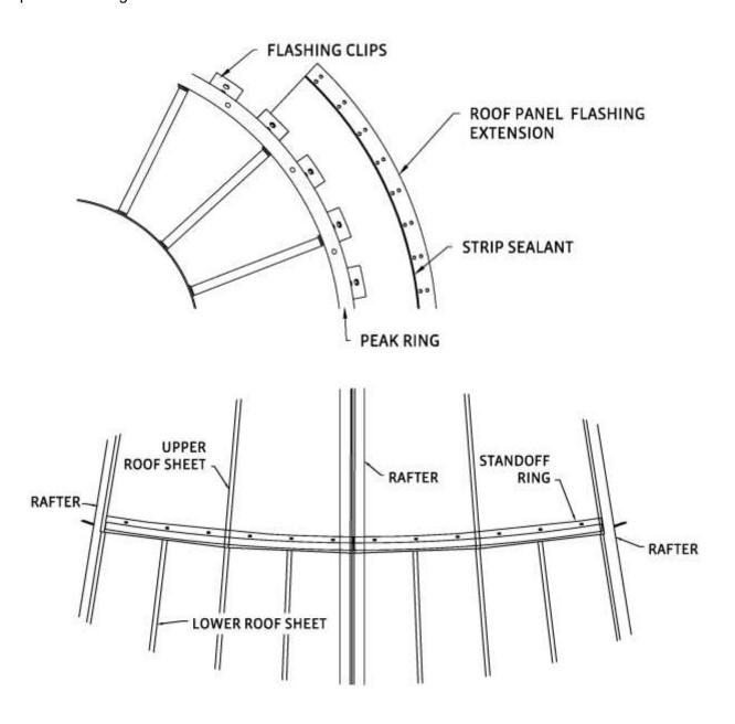
Install roof panels in a counter clockwise direction, always working to the right around the bin. Place sealant on the top right rib of the previously installed roof panel. Position the roof panel in a vertical position and lock the left rib of the current panel over the right rib of the previously installed panel. Slowly rotate the roof panel down.
