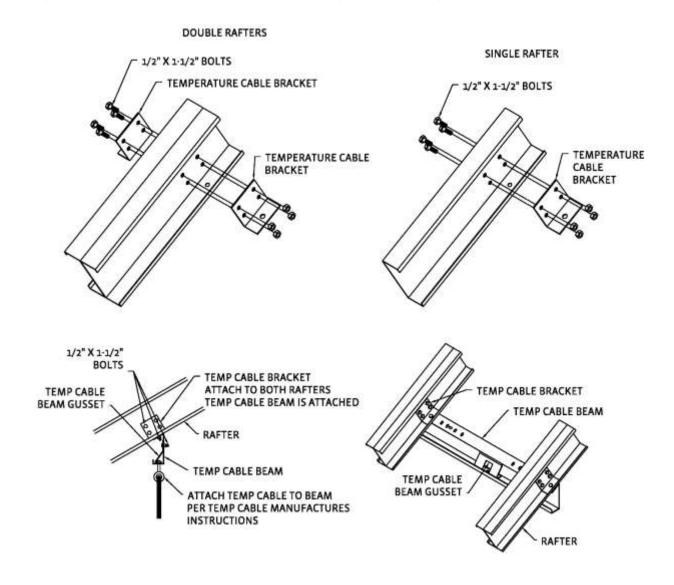
Once completed verify the temperature cable layout is identical to the following illustrations:
