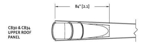
NOTE: DISTANCE SHOWN IS FROM BACK OF FAN TO BOTTOM OF UPPER ROOF SHEET. CB22, CB24 & CB26 BINS REQUIRE FAN TO BE INSTALLED ON 2 ROOF PANELS.
