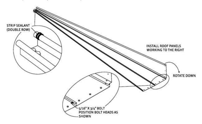
Continue the installation of the remaining roof panels as described previously. Align roof panel holes and tighten hardware as described previously. When the last roof panel is placed, it will have to be interlocked by using a rubber mallet. Starting at the top and working down the length of the panel, tap the vertical rib until it is locked to the other panel.
