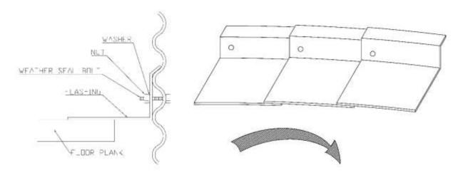
Continue to assemble the remaining floor planks and supports according to the appropriate support spacing instructions provided (bulletin 1050). On larger floors an individual row may be shipped with more than 1 plank to span the entire bin diameter. These floor planks are not of equal length to allow for offsetting of joints. Splices are used to secure the joints.
