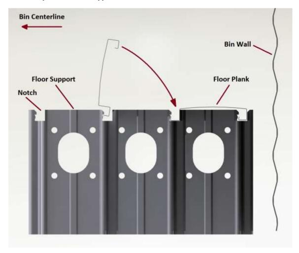
Continue to install the remaining floor planks and supports as described previously. Once you have installed 4-5 rows of floor planks, anchor the assembled floor section to the bin wall by installing several flashing sections as indicated in the following illustration to prevent movement of the floor.
