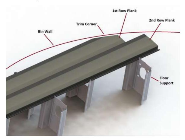
Locate the supports for row #2. These supports should be spaced as indicated in the layout instructions (bulletin 1050). Then holding the channel lock plank with the open J-section down, place the floor plank into the slot of the supports furthest from row #1 and after the floor plank is in contact with all supports, rotate the plank to row #1, and snap into place as shown in the following illustration.
