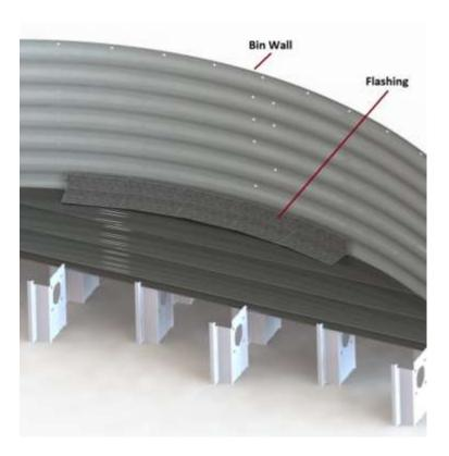
**Note**: Overlap the flashing so that the sweep auger wheel must climb up and over the leading edge of the following flashing piece. Wheel rotation follows the arrow in the illustration shown below.
