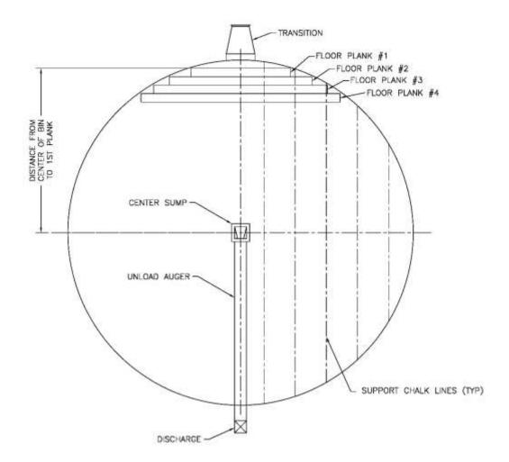
Locate the center of the bin. Chalk a line on the same centerline as the unloading auger. Refer to the appropriate floor support layout and create chalk lines on the concrete floor parallel to the bin centerline at the specified locations for the floor supports.
