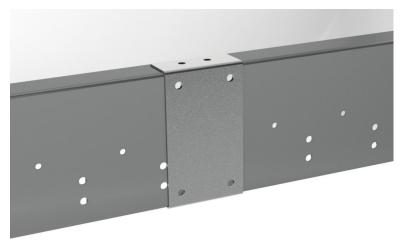
Bolt the floor bracing clips to the floor braces. These connections will require 1/2" x 1-1/2" (1.27cm x 3.81cm) Grade 5 bolts with lock washer and nut.
