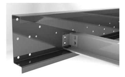
14' (4.26m) and 16' (4.87m) side channels require a bolted splice plate on the exterior of the side channel splice line. These connections will require 1/2" x 1-1/2" (1.27cm x 3.81cm) Grade 5 bolts with lock washer and nut. Bolt heads are to be located to the exterior of the platform.
