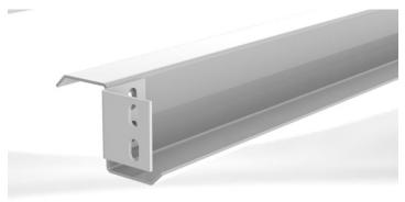
14' (4.26m) and 16' (4.87m) floor braces require a bolted splice plate on the bottom of the floor brace splice line. These connections will require 1/2" x 1-1/2" (1.27cm x 3.81cm) Grade 5 bolts with lock washer and nut.
