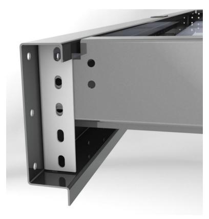
14' (4.26m) and 16' (4.87m) end channels require a bolted splice plate on the exterior of the end channel splice line. These connections will require 1/2" x 1-1/2" (1.27cm x 3.81cm) Grade 5 bolts with lock washer and nut. Bolt heads are to be located on the exterior of the platform.
