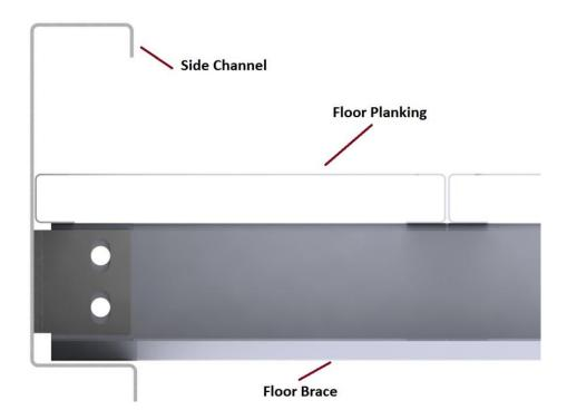
When positioned correctly there will be approximately 2-1/2" (6.35cm) minimum overlap on each end of the floor planking resting on the end channel frame. Floor planks must rest on the end channel ledge to provide adequate support. When positioned correctly there will be an approximate gap of 1/4" (.63cm) between edge of plank and the face of the end channel.
