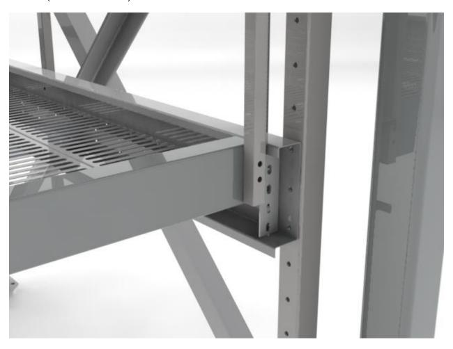
Position the handrail reinforcement strap across the end of the safety handrail to enclose and reinforce the corners. Fasten the strap to the handrail with (3) #10 self-drilling TEK screws on each side as required.
