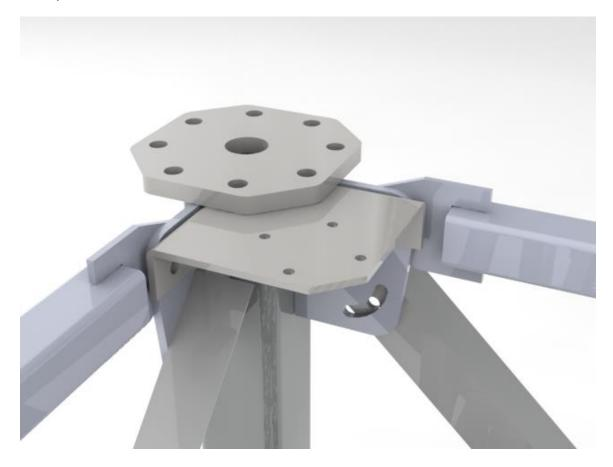
Align the single row of holes along the length of the adjustable post to the mounting holes in the side channel and bolt the adjustable post to the bracket. These connections will require 1/2" x 1-1/2" (1.27cm x 3.81cm) Grade 5 bolts with lock washer and nut.
