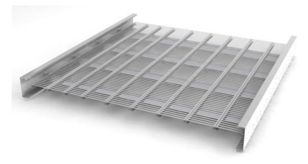
Bolt planking first to side channel and then successive planks to each other. These connections will require 3/8" x 1" (.95cm x 2.54cm) Grade 5 bolts with lock washer and nut.
