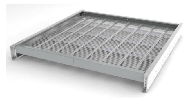
**Important Note**: Verify the orientation of the clips. The toe of the 5 slot clip is to the interior of the internal platform. Verify that the top of all channel frame pieces are flush along the top surface.
