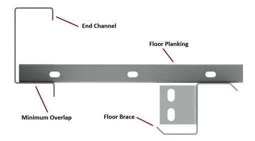
After positioning the floor planking correctly, screw the bottom side of the planking to the floor bracing using #10 self-drilling TEK screws as needed. On average each plank will require 4 screws equally spaced along each flange. Planking is to be field cut and positioned as required.
