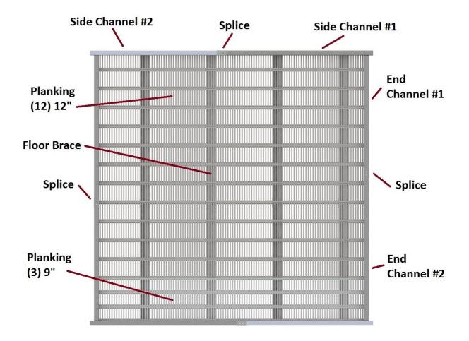
Determine which leg option will best suit the application. Floor bracing is to be positioned so as not to interfere with elevator legs and <u>cannot</u> be cut to fit. The floor bracing location can be adjusted in increments of 6.00" (15.24cm). If no elevator leg is required, equally space floor bracing in channel frame.
