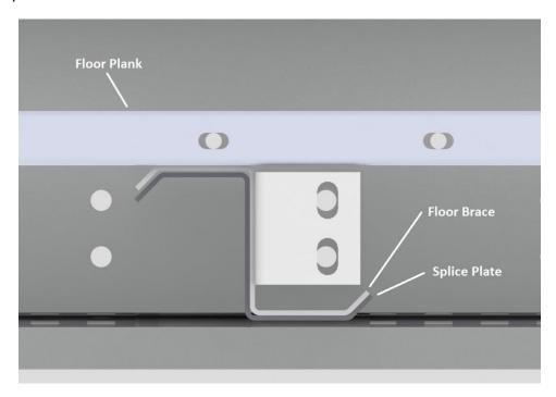
Position the floor bracing so as to not interfere with elevator leg. Bolt the floor bracing clips on the floor braces to the side channels. These connections will require 1/2" x 1-1/2" (1.27cm x 3.81cm) Grade 5 bolts with lock washer and nut.
