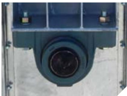
Pillow block bearings are used on both the head and boot and are either spherical or ball bearing design. The rugged shafts are of a minimum CR 1045 material.
