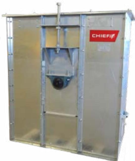
Bucket elevators also have urethane liners, easy-open hinged discharge inspection doors, and head hood slide clamps.
