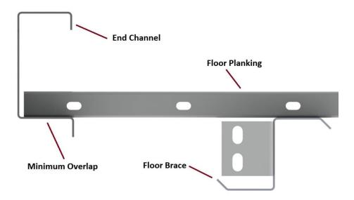
After positioning the floor planking correctly, screw the bottom side of the planking to the floor bracing using #10 self-drilling TEK screws as needed. On average each plank will require 4 screws equally spaced along each flange. Planking is to be field cut and positioned as required.
