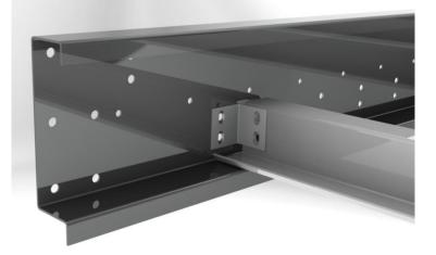
14' (4.26m) and 16' (4.87m) side channels require a bolted splice plate on the exterior of the side channel splice line. These connections will require 1/2" x 1-1/2" (1.27cm x 3.81cm) Grade 5 bolts with lock washer and nut. Bolt heads are to be located to the exterior of the platform.
