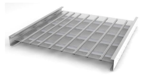
Bolt planking first to side channel and then successive planks to each other. These connections will require  $3/8^{\circ} \times 1^{\circ}$  (.95cm x 2.54cm) Grade 5 bolts with lock washer and nut.
