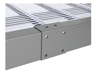
Install the adjustable posts inside the tower bay. Bolt the adjustable post mounting bracket on the tower column posts.
