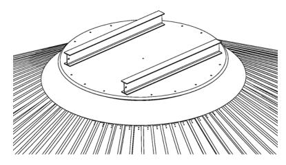
Place peak support posts on the 60" (152.4cm) support beams. Verify correct height position underneath catwalk as required. Cut peak support posts as needed to custom fit height required. Weld peak support posts to 60" (152.4cm) support beams using 1/4" (.63cm) fillet weld at all contact points.
