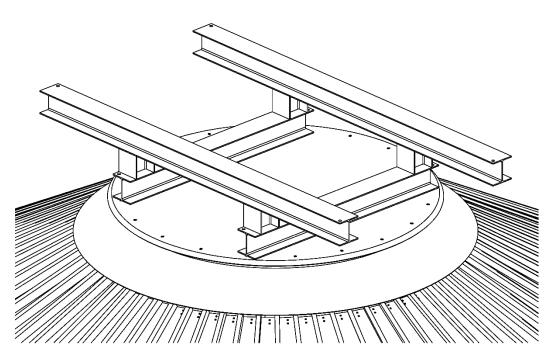
Next, install second set of 104" (264.1cm) support (spreader) beams on top of the first set of 104" (264.1cm) beams. The second set of 104" (264.1cm) support beams will run parallel to the installed catwalk and must contact the catwalk cross members only. Weld support beams using 1/4" (.63cm) fillet weld at all contact points.
