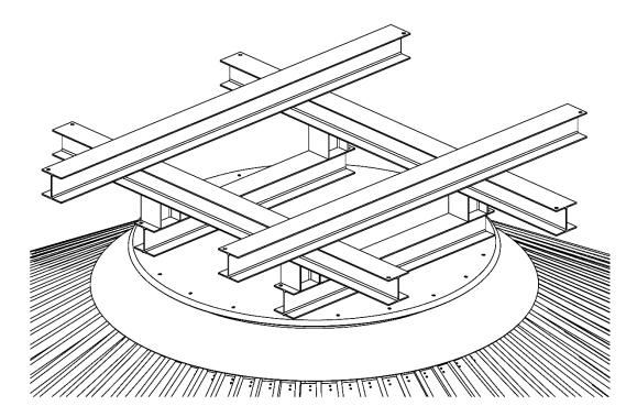
**Note**: Verify the correct placement of all items for correct beam mounting. The top illustration below shows the correct placement of the catwalk spreader beams below the truss sides. The bottom illustration shows the incorrect mounting of the catwalk spreader beams.
