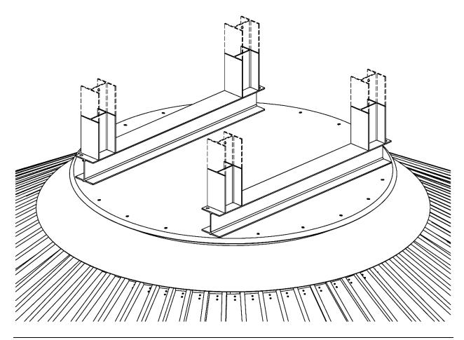
Install first set of 104" (264.1cm) support beams on top of the peak support posts. Verify correct height position underneath catwalk as required. First set of 104" (264.1cm) support beams will run perpendicular to the installed catwalk. Weld support beams using 1/4" (.63cm) fillet weld at all contact points.
