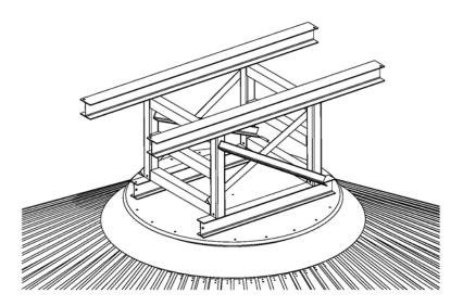
Next, install second set of 104" support (spreader) beams on top of the first set of 104" beams. The second set of 104" support beams will run parallel to the installed catwalk and must contact the catwalk cross members only. Weld support beams using ½" fillet weld at all contact points.
