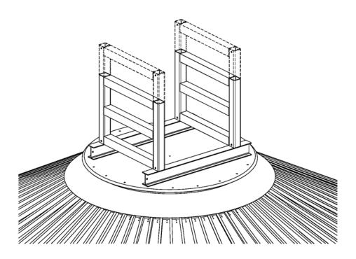
Install diagonal bracing on the peak support sides. Cut diagonal braces to length and weld two diagonal braces to each side of peak support side (four diagonal braces total). One diagonal brace on the outside face of each peak support side and one on the inside face connecting the two support sides. Weld diagonal bracing to peak support sides using ¼" fillet weld at all contact points.
