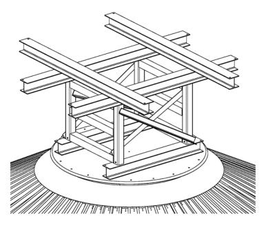
**Important Note**: Verify the correct placement of all items for correct beam mounting. The top illustration below shows the correct placement of the catwalk spreader beams below the truss sides. The bottom illustration shows the incorrect mounting of the catwalk spreader beams.
