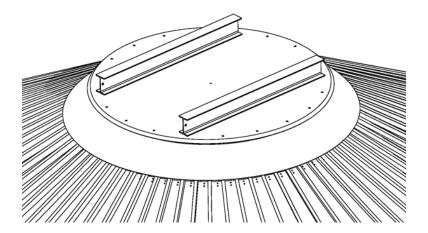
Place peak support sides on the 60" support beams. Verify correct height position underneath catwalk as required. Cut peak support sides as needed to custom fit height required. Weld peak support sides to 60" support beams using  $\frac{1}{4}$ " fillet weld at all contact points.
