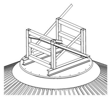
Install first set of 104" support beams on top of the peak support sides. Verify correct height position underneath catwalk as required. First set of 104" support beams will run perpendicular to the installed catwalk. Weld support beams using  $\frac{1}{4}$ " fillet weld at all contact points.
