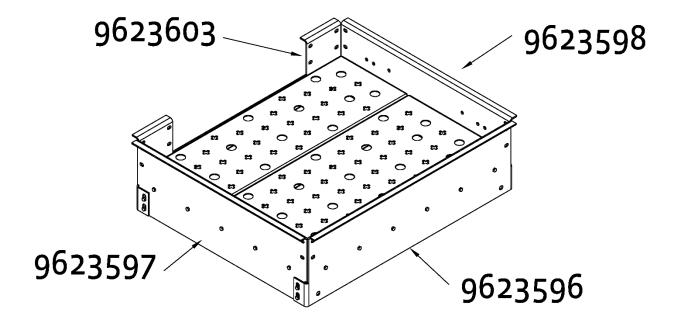
Assemble horizontal mounting brackets to the exterior of the toeboard and the ladder base mounting bracket to the inside of the toe board using 3/8" X 1.0" (.95cm x 2.54cm) bolts.
