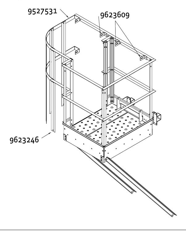
Assemble and install the support bracing located beneath the ladder platform as shown in the following illustration. Attach the kicker brace with the clamps installed around the tower post using 1/2" x 1.25" (1.27cm x 3.17cm) bolts. The kicker brace is positioned between the tower bay x-bracing, with the platform bracing attached to the kicker brace.
