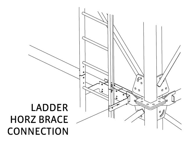
The standoff bracket connection is required to attach the ladder to the horizontal brace bracket. Attach the standoff bracket as shown in the following illustration.
