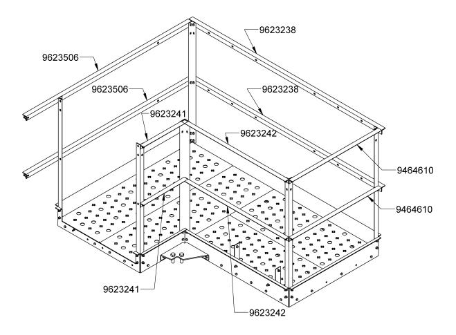
Assemble the brace supports to the underside of the platform floor planks as shown in the following illustration using 3/8" X 1.0" (.95cm x 2.54cm) bolts.
