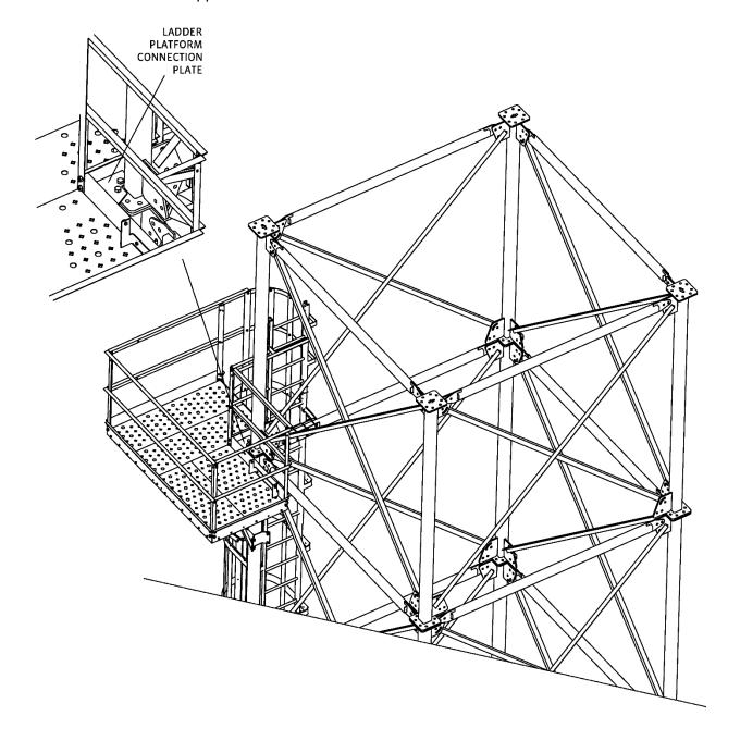
Assemble and install the support bracing located beneath the ladder platform. Attach the bracing mounts around the tower post using 1/2" x 1.25" (1.27cm x 3.17cm) bolts.
