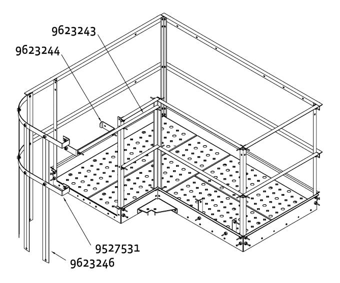
Verify the platform location on the completed tower as described in the project specific engineering drawings supplied for the project or the <u>standard platform locations</u> if applicable. Connect the assembled platform to the completed tower at the tower post endplate location, using the post connection hardware supplied with the tower.
