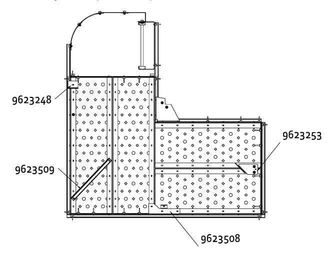
Assemble the platform ladder support and cage as shown in the following illustration using 3/8" X 1.0" (.95cm x 2.54cm) bolts.
