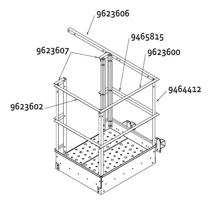
Assemble the platform ladder support and cage as shown in the following illustration using 3/8" X 1.0" (.95cm x 2.54cm) bolts.
