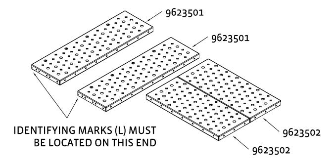
Assemble toe boards to the floor planks using 3/8" X 1.0" (.95cm x 2.54cm) bolts and the tower attachment plate to the corner of the toe board as shown in the following illustration.
