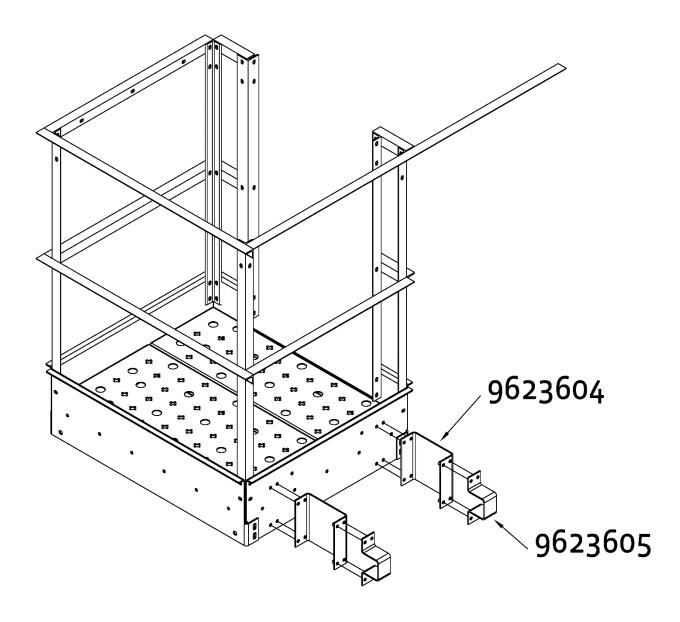
Assemble posts to the inside of the toe boards using 3/8" X 1.0" (.95cm x 2.54cm) bolts. Assemble safety rails to the posts using 3/8" X 1.0" (.95cm x 2.54cm) bolts.
