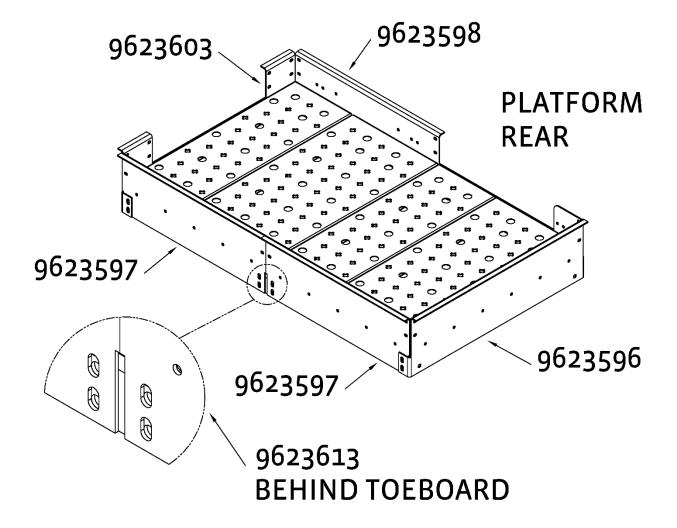
Assemble horizontal mounting brackets to the exterior of the toeboard and the ladder base mounting bracket to the inside of the toe board using 3/8" X 1.0" (.95cm x 2.54cm) bolts.
