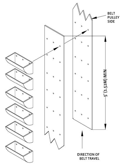
**Important Note**: Recheck all bolts in the belt and buckets for proper tension. All bolt heads are to be flush with the belt surface. Replace cleanout doors, inspection section back panel, screen door front panel, & head hoods.
