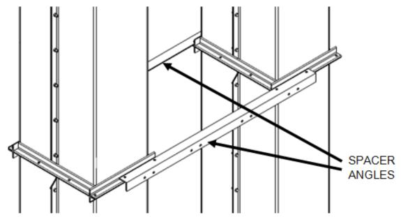
For CBEG48-50, spacers are placed between the lower and upper ends of each pair of legs to hold the sections parallel and a brace set diagonally on each spacer set for support.
