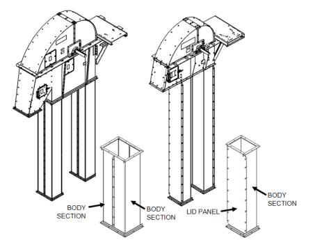
**Important Note**: When attaching leg sections that consist of a body section and lid panel, verify that the lid panel is located away from the center of the elevator.
