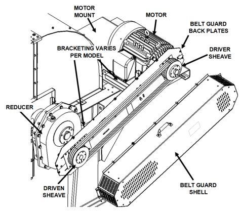
**Important Note:** Do not operate the bucket elevator without a correctly installed belt guard assembly.
