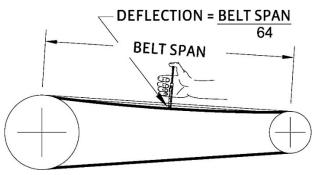
**Important Note**: Compare the force you have applied with the values in the following chart. The force should be between the minimum and maximum shown. The maximum value shown is for a "New Belt", and new belts should be tensioned at this value to allow for expected tension loss. Used belts should be maintained at the minimum value.
