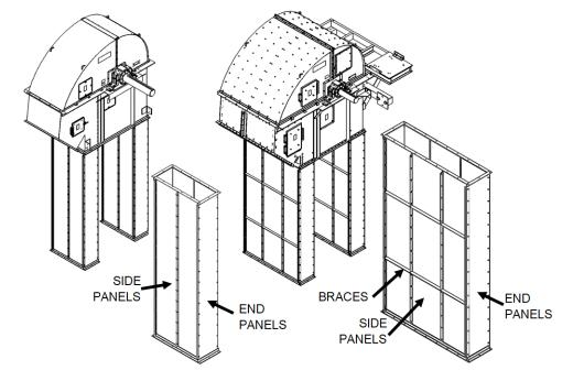
Align the flanges on the leg sections and place spacer angles between the lower ends of each pair of leg sections to hold the sections parallel and help reduce flange stress while making the horizontal assembly.
