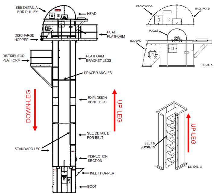
The general installation of the bucket elevator components will be in the following order. The elevator can be completely assembled within about 10' of the ground if this method is used. Crane time can be reduced if 30' sections, including accessories, are attached horizontally on the ground, and then hoisted with the crane. Refer to unit customer drawings for stacking order.
