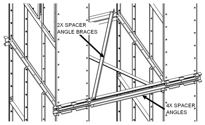
When installing explosion vented leg sections, shipping fasteners must be removed and explosion relief fasteners installed as shown in the following illustration.
