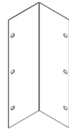
HOPPER STARTER FLASHING
